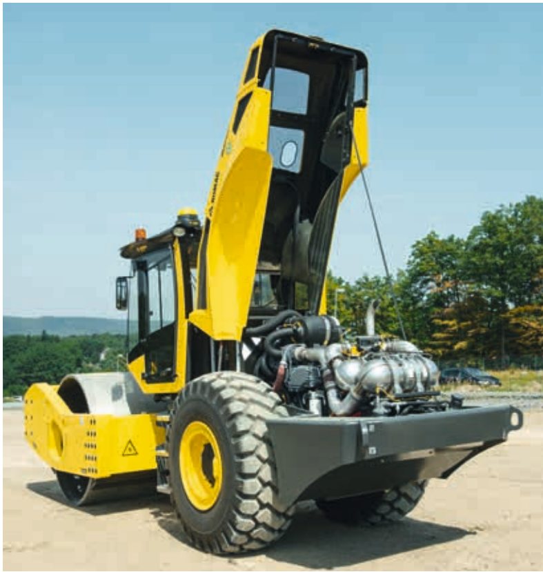
Handy, large, hinged cover: all service points are easily accessible.
