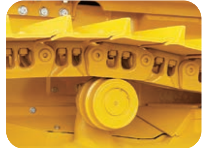
Individual links can be replaced with common track tools
